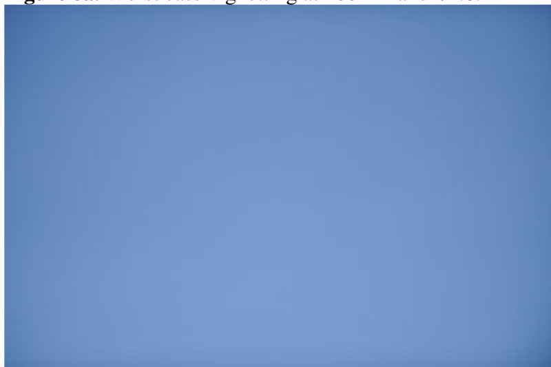
Figure 8a. Worst case vignetting at 200mm and f/2.8.
